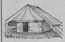
Double fly: four folds of cloth throughout Kanat 6 ft. high, having semicircular saibans at the ends, the rear one is enclosed by a wall 6 ft. high to form a Bath Room, when verandah enclosed with chicks, form a convenient Office Room, the side saibans give an ample space for servants and luggage etc. complete with durrie (for Centre Room only) chicks, purdahs, gunny bags and mallet etc.
