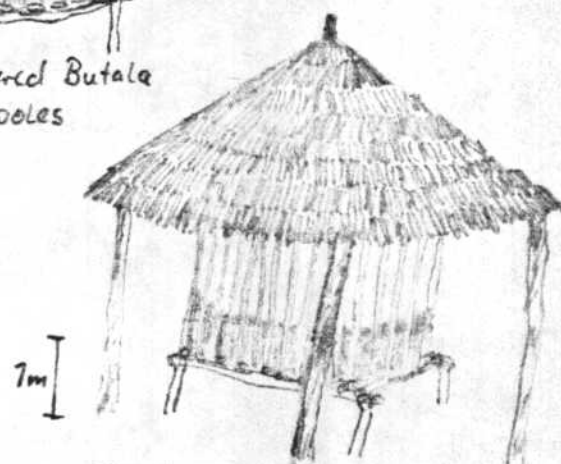
Fig. 4 Butala bin from wooden poles, partly plastered from inside with big roof providing Veranda
