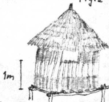
Fig. 3 Partly plastered Butala of wooden poles
